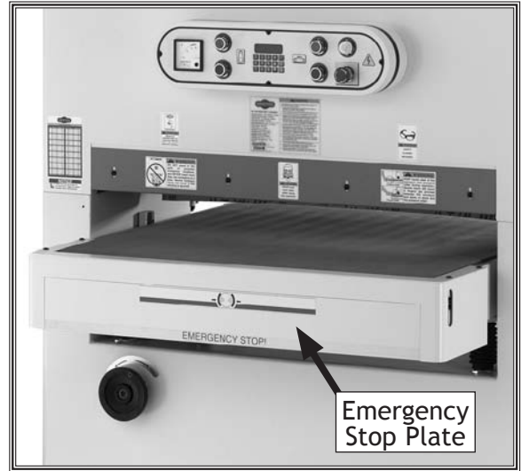
Figure 19. Emergency stop plate.
